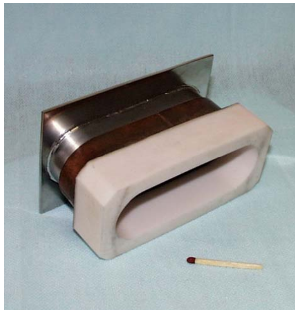
Figure 8: Al_2O_3 ceramic brazed with austenitic steel with copper layer according to Type II
